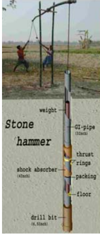
Stonehammer drilling is suitable for hard soils.
